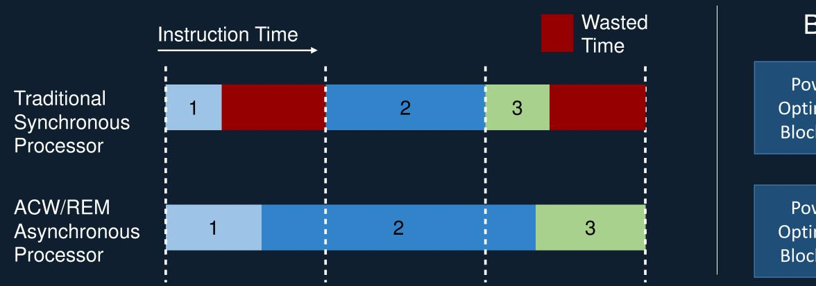
Relaxing timing constraints allow some instructions to take longer On average, computational performance does not change Smaller logic blocks are more power and area efficient
